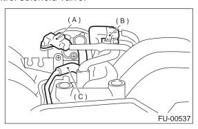
7) Disconnect throttle position sensor connector.
