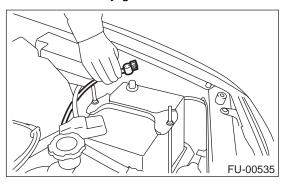
Remove air intake chamber. <Ref. to IN(H6DO)-6, REMOVAL, Air Intake Chamber.>
