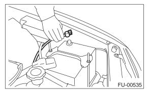
2) Disconnect connector (A) from idle air control solenoid valve.
