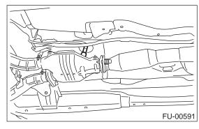
3) Connect connector to rear oxygen sensor.
