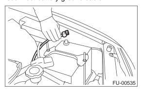
2) Disconnect connector from rear oxygen sensor.
