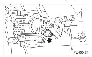
4) Remove fuel pump relay from mounting bracket.
