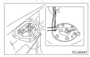
(2) Connect connector from fuel sub level sensor.
