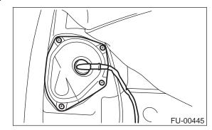
9) Disconnect connector from fuel sub level sensor.
