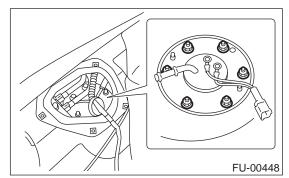
12) Drain fuel from fuel tank by using hand pump.
