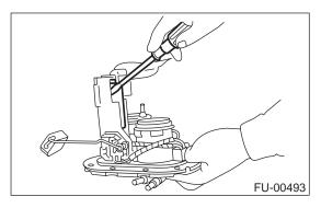
2) Disconnect connector from fuel pump.
