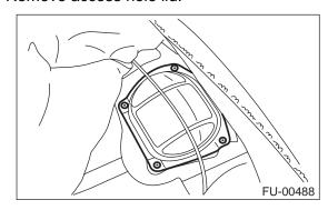
10) Disconnect connector from fuel pump.
