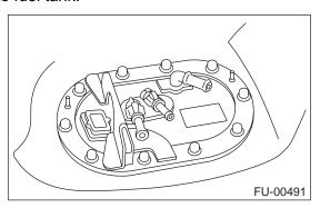
14) Take off fuel pump assembly from fuel tank.
