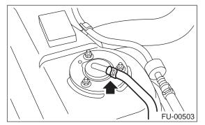
3) Remove bolts which install fuel cut valve.
