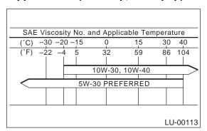
The proper viscosity helps vehicle get good cold and hot starting by reducing viscous friction and thus increasing cranking speed.
