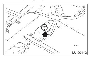
5) Fill engine oil through filler pipe up to upper point on level gauge. Make sure that vehicle is placed level when checking oil level. Use engine oil of proper quality and viscosity, selected in accordance with the table in figure.
