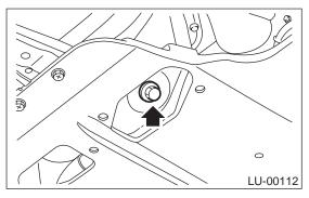
2) Open engine oil filler cap for quick draining of the engine oil.
