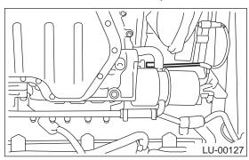
6) Remove oil pressure switch.
