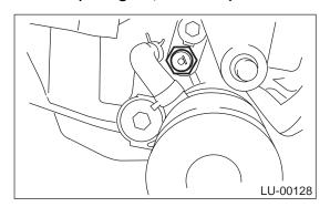
3) Connect terminal of oil pressure switch.
