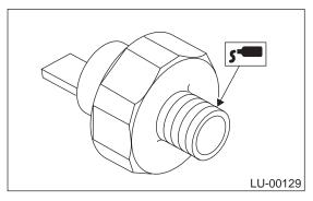
2) Install oil pressure switch.
