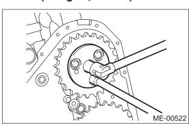
2) Install timing chain assembly. <Ref. to ME(H6DO)-42, INSTALLATION, Timing Chain Assembly.>
