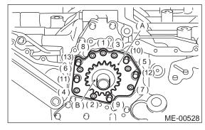
10) Install camshaft sprocket. <Ref. to ME(H6DO)-46, INSTALLATION, Camshaft Sprocket.>
