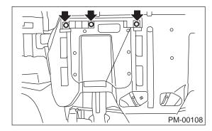
3) Remove oil filter with ST. ST 498547000 OIL FILTER WRENCH
