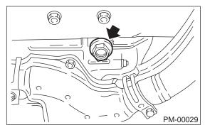
2) Reinstall drain plug after draining gear oil and tighten it to the specified torque.
