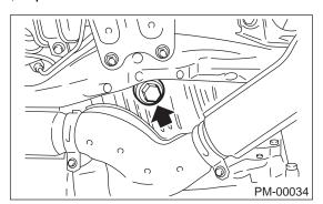
2) Reinstall drain plug after draining differential gear oil and tighten it to the specified torque.
