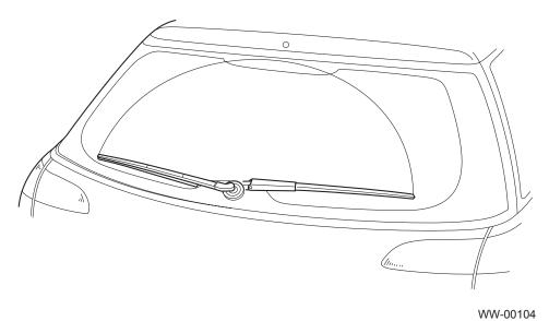
3) The wiper blade is attached to the arm by means of a U-hook joint in the same way as with the front wipers.
