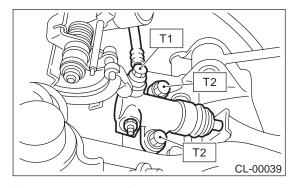
3) After bleeding air from the operating cylinder, ensure that clutch operates properly. <Ref. to CL-20, Clutch Fluid Air Bleeding.>
