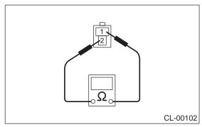
Clutch switch (With cruise control)
