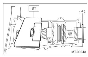
(A) Adjust clearance to zero without shim.
