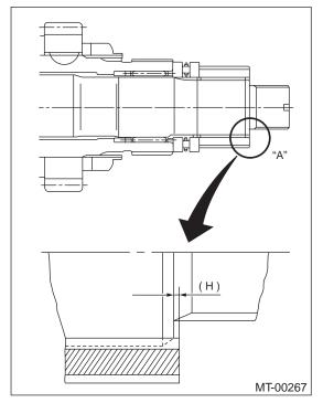
2) Using ST1, ST2 and ST3, tighten lock nut to the specified torque.
