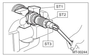
2) Withdraw drive pinion from driven shaft. Remove differential bevel gear sleeve, adjusting washer No. 1, adjusting washer No. 2, thrust bearing, needle bearing, drive pinion collar, needle bearing and thrust bearing.
