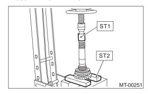
11) Remove sub gear for 1st driven gear.
