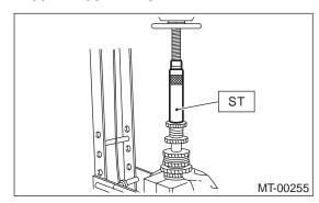
7) Install a set of roller bearings onto the driven shaft using ST and press.
