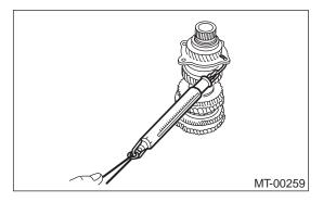
12) Install roller bearing onto drive pinion.
