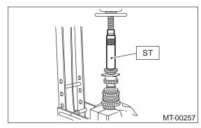
9) Install lock washer. Install lock nut and tighten to the specified torque using ST.
