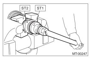
5) Remove 5th driven gear using ST. ST 499857000 5TH DRIVEN GEAR REMOV-
