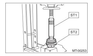
5) Install 2nd driven gear, inner baulk ring, synchro cone, outer baulk ring and insert onto driven shaft.
