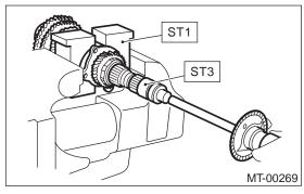
4) If starting torque is not within specified limit, select new adjusting washer No. 1 and recheck starting torque.
