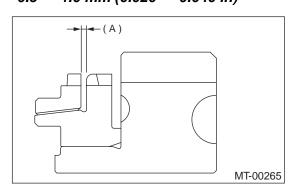
When the contact surface of the synchronizer ring insert is scored or abnormally worn down.
