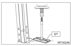
4) Straighten lock nut at staked portion. Remove the lock nut using ST1 and ST2.
