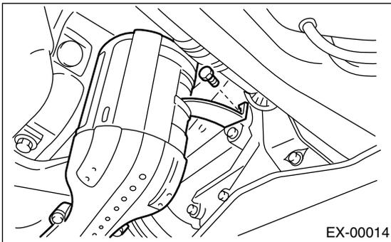
8) Tighten the bolt which holds the center exhaust pipe to hanger bracket.
