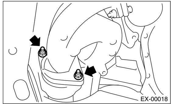
7) Remove the center exhaust pipe. <Ref. to EX(H4DOTC)-9, REMOVAL, Center Exhaust Pipe.>
