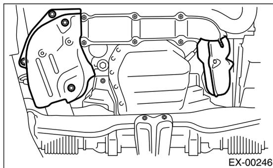
6) Remove the nuts and bolts which hold the front exhaust pipe assembly to turbocharger joint pipe.
