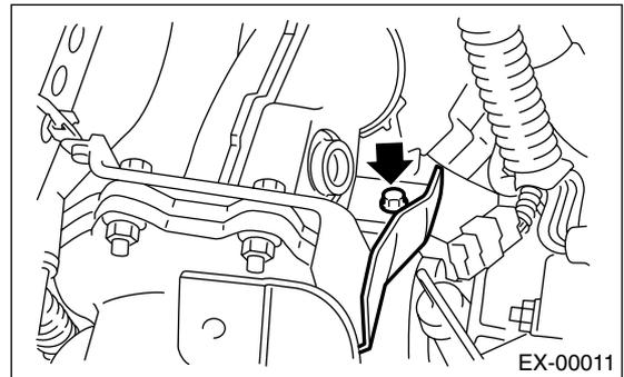
11) Place the turbocharger upper cover, and tighten the bolts which install the upper side of upper cover.
