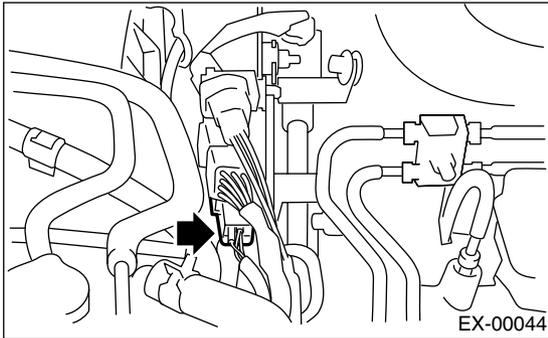
3) Remove the front oxygen (A/F) sensor. <Ref. to FU(H4DOTC)-38, REMOVAL, Front Oxygen (A/F) Sensor.>
