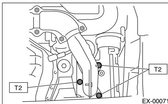
6) Install the upper and lower exhaust manifold covers (LH).
