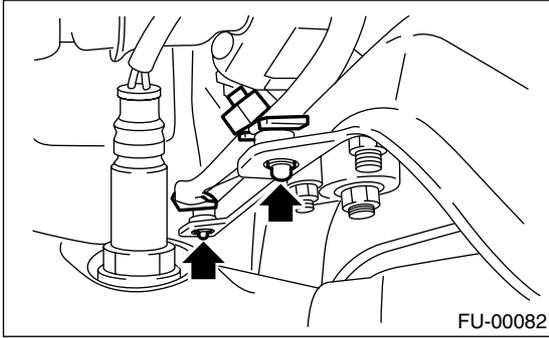
7) Tighten the bolt which holds the center exhaust pipe bracket to transmission.
