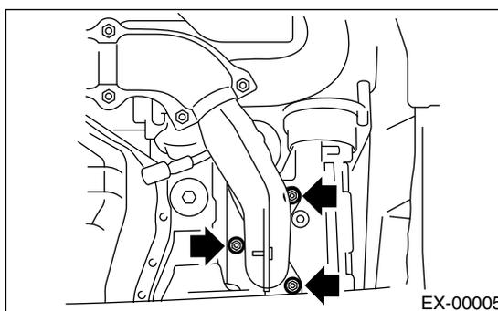
8) Remove the front exhaust pipe assembly.
