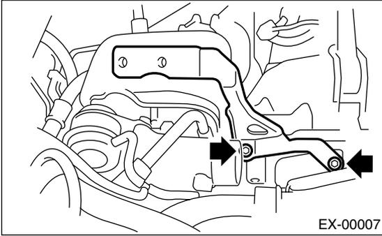
17) Install the intercooler. <Ref. to IN(H4DOTC)-11, INSTALLATION, Intercooler.>
