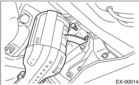
17) Remove the intercooler bracket.
