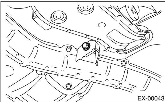
19) Remove the center exhaust pipe.
