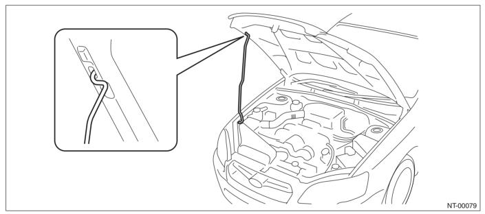
• WHEN WIDER HOOD OPENING IS NECESSARY Set the stay into the hole of lower hood as shown in the figure below.
