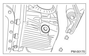
2) Replace the gasket with new part, and then tighten the drain plug to specified torque.
