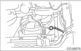
8) Disconnect the radiator outlet hose from thermostat cover.
