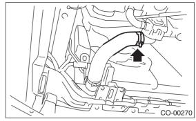
9) Disconnect the ATF cooler hoses from ATF pipes. (AT model)
