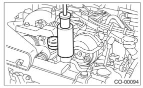
2) In the following cases, apply a pressure of 157 kPa (1.6 kg/cm<sup>2</sup>, 23 psi) to the radiator.
