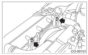
11) Remove the radiator sub fan motor assembly from underneath the vehicle.
