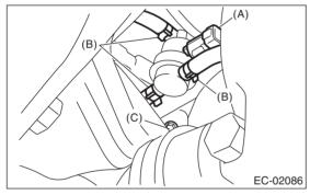
7) Remove the pressure control solenoid valve from the bracket.
