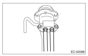
3) Remove the shut valve from the fuel filler pipe.
