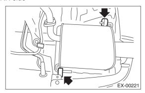
3) Remove the front and rear cushion rubbers, and then remove the muffler.
