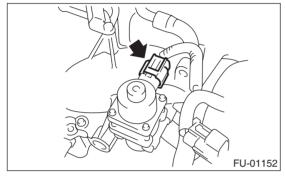
3) Remove the EGR valve from intake manifold.
