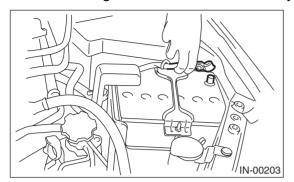
2) Remove the clip fastening the harness and disconnect the rear oxygen (A/F) sensor connector.
