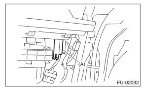
4) Disconnect the connector from fuel pump relay.
