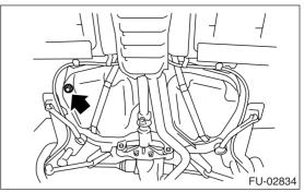
7) Tighten the fuel drain plugs.
