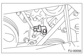
14) Disconnect the connector from power steering pump switch (A).
