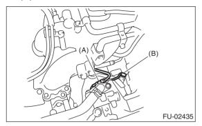
16) Disconnect the connector from camshaft position sensor.
