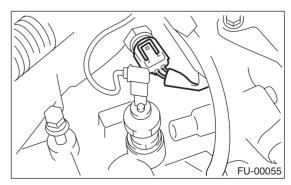
10) Connect the PCV hose (A) to intake manifold.
