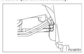
4) Connect the fuel injector pipe RH to the fuel pipe.
