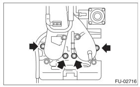
20) Remove the intake manifold.
