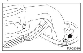
12) Remove the bolts which hold engine harness to intake manifold.
