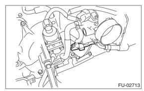
9) Connect the connector to engine coolant temperature sensor.
