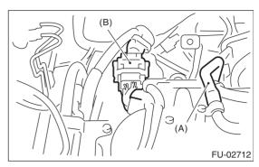
11) Disconnect the connectors from the engine coolant temperature sensor.
