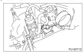
13) Disconnect the connector from crankshaft position sensor.
