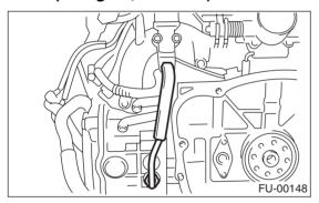
4) Connect the connectors to camshaft position sensor.
