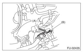
7) Connect the connector to crankshaft position sensor.
