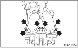
2) Tighten the bolts which install fuel pipes on intake manifold.
