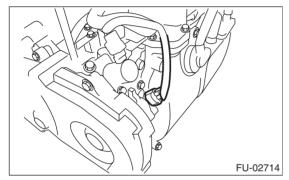
17) Remove the EGR pipe from intake manifold.
