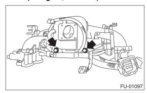
9) Hold the engine harness using the harness band clips.
