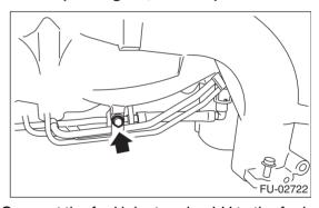
3) Connect the fuel injector pipe LH to the fuel pipe.
