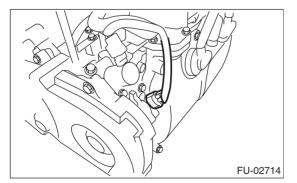
5) Connect the connector to the power steering pump switch (A).
