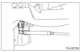
17) Disconnect the quick connector that fastens the fuel injector pipe LH to the fuel pipe.
