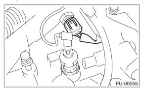
4) Remove the engine coolant temperature sensor.
