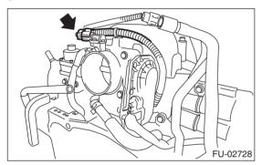
3) Remove the manifold absolute pressure sensor from throttle body.
