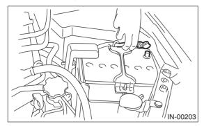
2) Disconnect the connector from manifold absolute pressure sensor.
