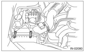
4) Pull the air cleaner case (rear) backward of the vehicle, and remove the air cleaner element.
