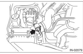
3) Remove the clip (A) securing upper side of air cleaner case.
