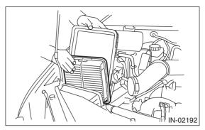
7) Remove the bolts (A) and nut (B) which secure the air cleaner case to body.
