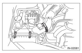
6) Remove the air cleaner case (rear) and air cleaner element.
