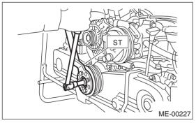
3) Check that the tightening angle of the clamp pulley bolt is a minimum of  $65^{\circ}$ Perform the following procedures when less than  $65^{\circ}$ .
