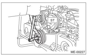
3) Remove the crank pulley.
