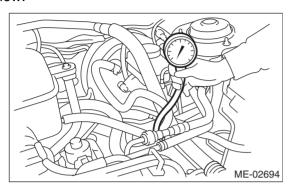
Vacuum pressure (at idling, A/C "OFF"): -60.0 kPa ( -450 mmHg, -17.72 inHg) or less
