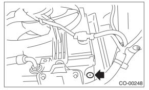
4) Install the drain plug.
