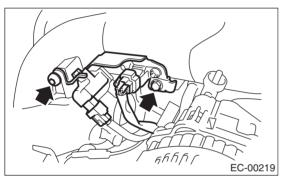
4) Disconnect the connector from purge control solenoid valve.
