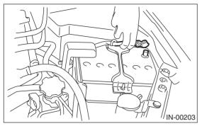
3) Remove the solenoid valve bracket assembly from intake manifold.
