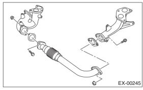
2) Install the front exhaust pipe cover.
