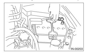
3) Disconnect the exhaust temperature sensor connector.
