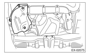
7) Remove the nuts which hold the front exhaust manifold to joint pipe.
