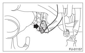
5) Disconnect the engine coolant hoses from throttle body.
