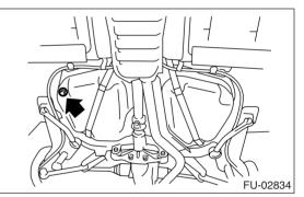
7) Tighten the fuel drain plugs.
