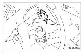
6) Remove the engine coolant temperature sensor.
