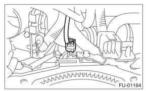
5) Remove the knock sensor from the cylinder block.
