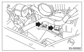
6) Remove the spark plug with a spark plug socket.
