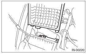
**C: INSPECTION** Replace if excessively damaged or dirty.
