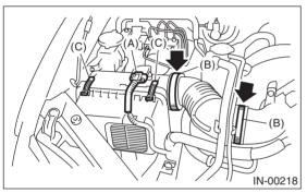
5) Remove the air cleaner case (rear) and air intake boot.
