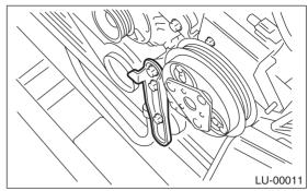
11) Remove the crankshaft position sensor.
