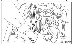
13) Remove the water pump. <Ref. to CO(H4DOTC)-15, REMOVAL, Water Pump.> 14) Remove the timing belt guide.
