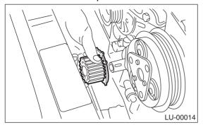
16) Remove the bolts which install oil pump onto cylinder block.
