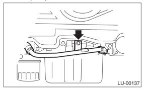
6) Remove the water pipe and hoses between oil cooler and water pump.
