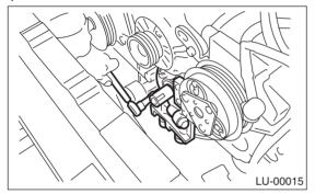
17) Remove the oil pump by using flat tip screwdriver.
