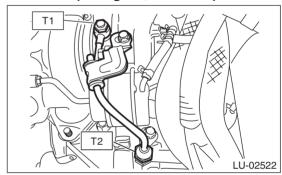
13) Tighten the bolts which hold the oil inlet pipe stay to the turbocharger.
