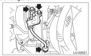
12) Tighten the union screws and flare nuts which secure the oil inlet pipe to the turbocharger.
